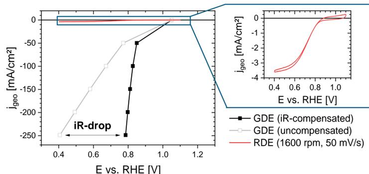
Fig. 2: ORR on GDE with 0.3 mg/cm<sup>2</sup> Pt/C (40 wt.-%) on Sigracet 29 BC MPL/GDL (black) and RDE with same catalyst loading (red).
