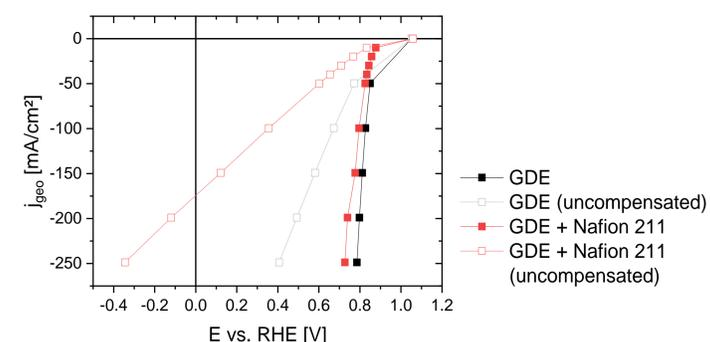
Fig. 4: ORR on GDE with 0.3 mg/cm<sup>2</sup> Pt/C (40 wt.-%) with (red) and without (black) hotpressed Nafion® 211.
