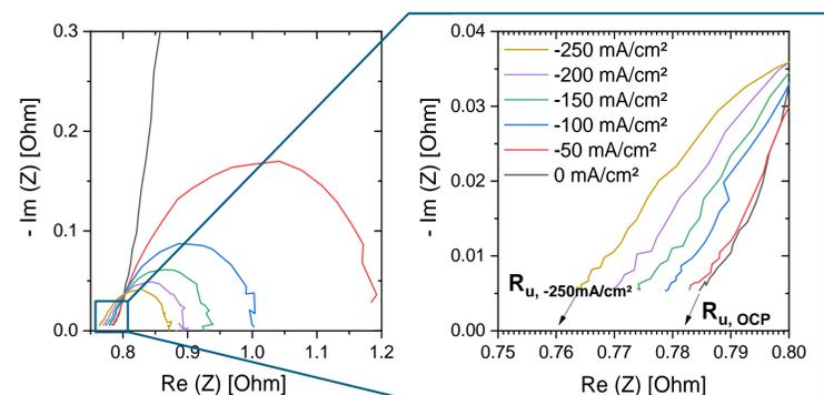
Fig. 3: Impedance measurements (1 kHz – 0.5 Hz) to determine uncompensated resistance (R<sub>u</sub>) at different current densities.
