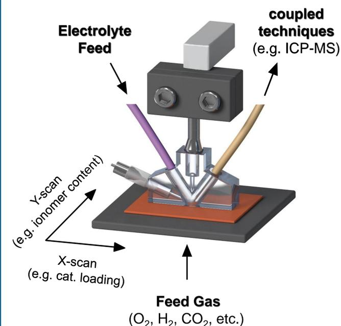
Fig. 5: Scheme of a Scanning Flow Cell (SFC).
