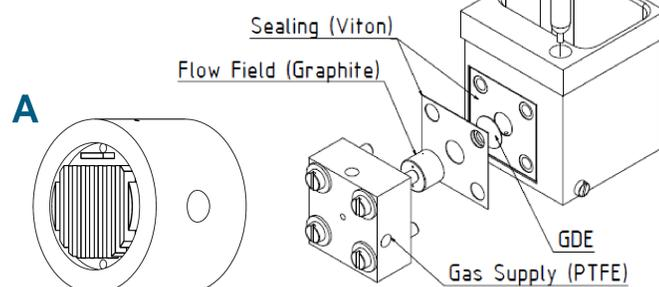
Fig. 1: Scheme of GDE set-up (B) and flow field (A).
