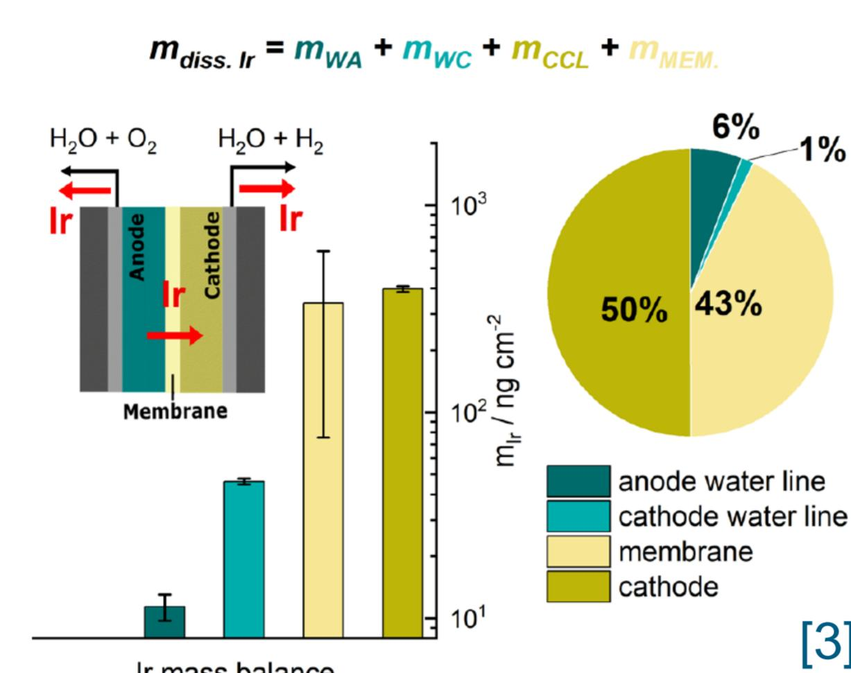
Activity and dissolution stability of Ir/Ru electrocatalysts tested in a model PEMWE
