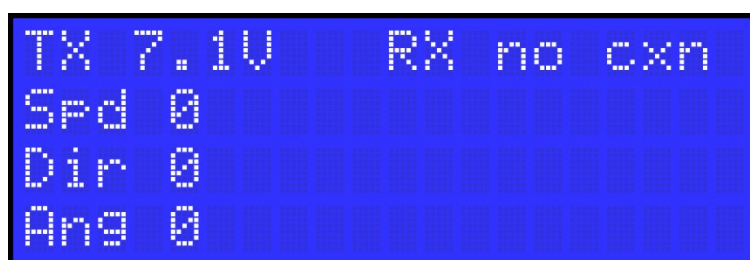
Figure 14: Connection warning in the LCD screen of the remote control. “no cxn” on the right indicates that the remote control is not connected to HydroBot.
